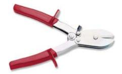
The blades inter-penetrate to form a fold on the periphery of the pipe, reducing its diameter, and allowing consistent slotted joints to be easily formed in all types of pipe (smoke and gas, extraction, ventilation, dust extraction, rainwater downpipes, etc.) Accurate adjustment is obtained by varying the pressure on the handles. - Insulating polypropylene grips. - Case-hardened blades and pins.
